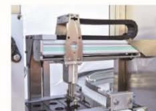
成品输出到输送带 Grab out and put on belt
