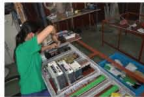
模块化电器组装 Module assembling for electric
