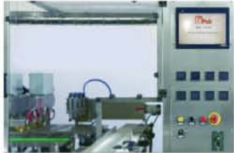
触摸屏人机交互 Touchscreen interface (PLC upon OMRON platform)
