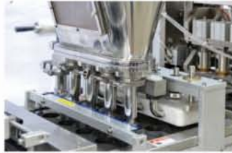
伺服驱动高精度灌装 Servo motor driven filler (Electric upon Schneider system)
